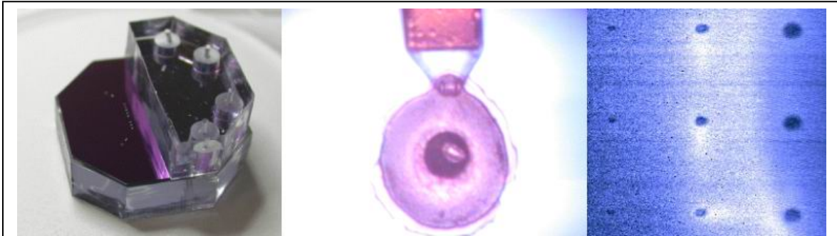
Fabricated inking chip with 4 reservoirs (left). A SPCP probe is being inked by contact (middle). Ten seconds, 30 seconds, and 1 min of contact printing resulted in patterns in the sizes of 600 nm, 1.3 \mu\text{m} , and 1.8 \mu\text{m} (right).
