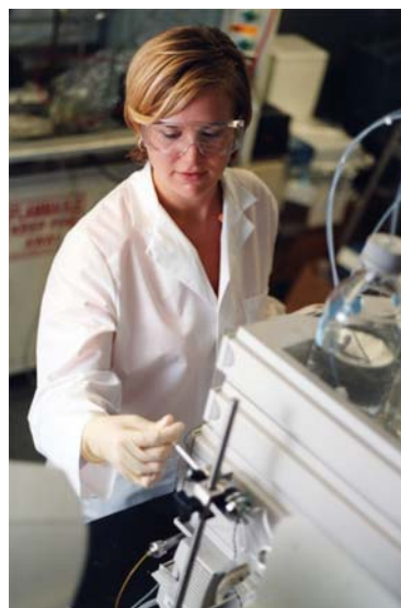
Jennifer Clery, a teacher at Evanston Township High School injecting DNA sample into HPLC for purification as part of her research project in the NU-NSEC 2002 RET program.
